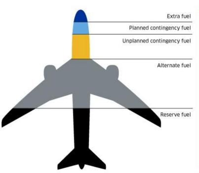
Extra fuel: Fuel which allows the aircraft to deviate from the planned route to avoid weather.
