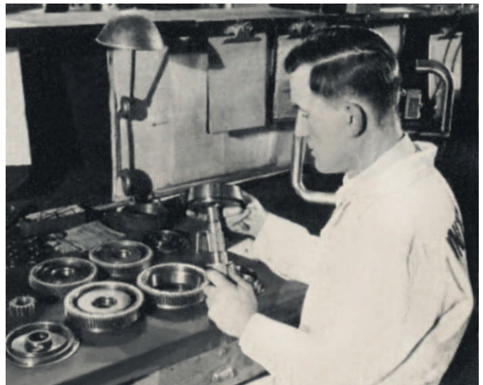
A Shop Inspector, one of many at the SFO Maintenance Base, tests and examines parts. Here he is checking a processed clutch assembly from one of the DC-6s four Wasp engines.
