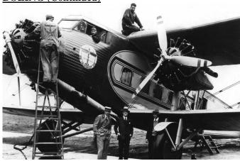
While Bill Boeing was pleased with the success of Boeing Air Transport and the Model 40A, he realized a larger airplane was necessary to be competitive with the Ford Tri-motor and other passenger-carrying aircraft. The result was the Boeing "Model 80". The first "80" was delivered to Boeing Air Transport (BAT) in August of 1928 and was immediately put into service on the San Francisco to Chicago CAM 18 route.
