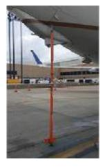
Ground Service Equipment Maintenance is deploying 475 tail stands to hubs and stations starting this month to support the aft ends of Boeing 737-900 and -900ER aircraft while parked at the gate to enable immediate deplaning of customers from the front of the plane.
