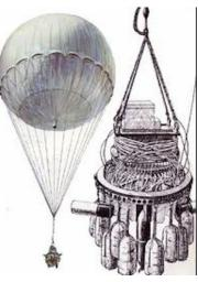
A unique lightweight system was needed to control the balloon. The balloon would be subjected to day and night temperature variations, causing the balloon to gain or lose altitude. A large ring would be attached to the balloon. On this ring were a number of sand bags, small battery, series of tiny explosives and a simple device that would could sense
